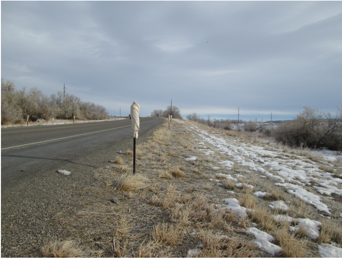
Figure 4. Wildlife-warning reflectors covered with white canvas bags in the reflectors-exposed versus covered with white bags experiment.
